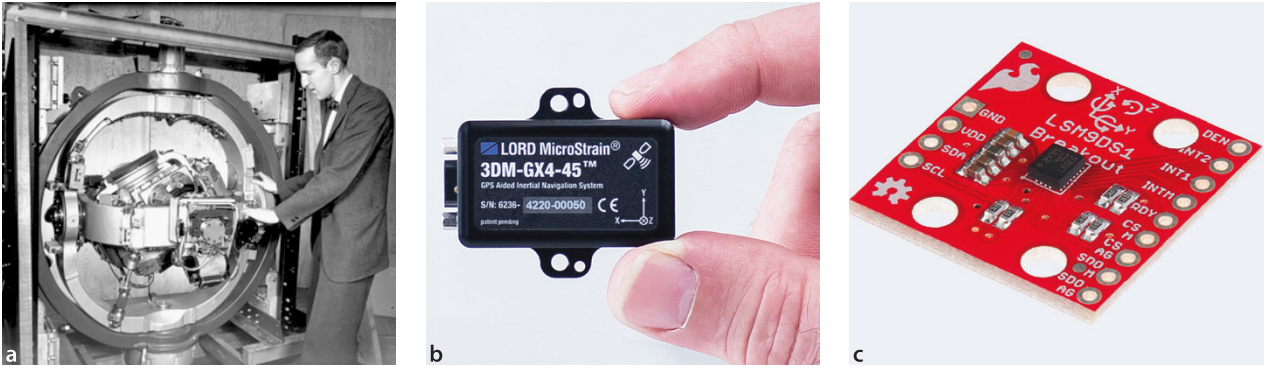
Fig. 3.9. a SPIRE (Space Inertial Reference Equipment) from 1953 was 1.5 m in diameter and weighed 1200 kg. b A modern inertial navigation system the LORD MicroStrain 3DM-GX4-25 has triaxial gyroscopes, accelerometers and magnetometer, a pressure altimeter, is only 36 \times 24 \times 11 mm and weighs 16 g (image courtesy of LORD MicroStrain); c 9 Degrees of Freedom IMU Breakout (LSM9DS1-SEN-13284 from SparkFun Electronics), the chip itself is only 3.5 \times 3 mm
