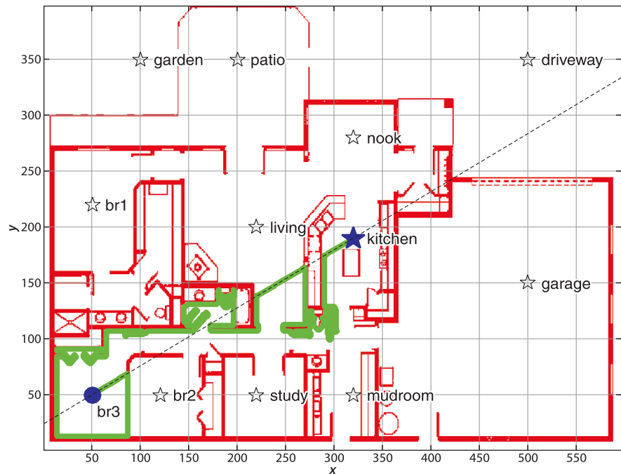
Fig. 5.4. Obstacles are indicated by red pixels . Named places are indicated by hollow black stars . Approximate scale is 4.5 cm per cell. The start location is a solid blue circle and the goal is a solid blue star . The path taken by the bug2 algorithm is marked by a green line . The black dashed line is the m-line, the direct path from the start to the goal
