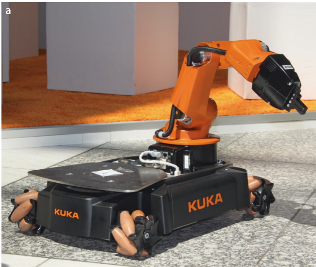
Fig. 4.18. a Kuka youBot, which has four mecanum wheels (image courtesy youBot Store); b schematic of a vehicle with four mecanum wheels in the youBot configuration
